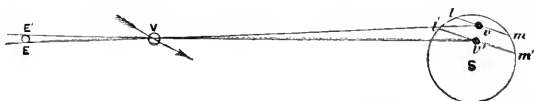
FIG. 13.—Illustrating the general principles on which the determination of the Sun's distance by transit observation depends.
